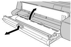
**2** Rotate the roll holder in the direction shown in the illustration so you can see the leading edge of the roll, then cut the media at the buckle.
